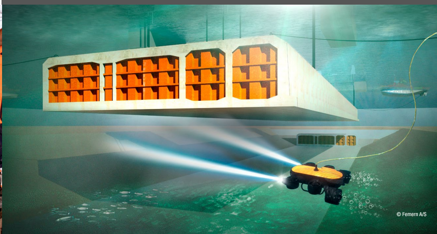
Lowering and connecting the tunnel elements
