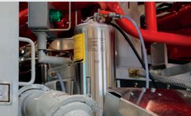
Spray tank with compressed air connection for easy cleaning of the hopper by moistening with release agent beforehand The central grease lubrication system on the boom reduces the time for daily maintenance
