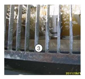
The example (3) shows heavy leaks between the wear ring and spectacle plate as well as between the S tube and wear ring. This provides clear information about worn out wear parts, defective thrust ring, or wrong installation.
